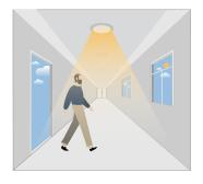
当检测到运动时, 灯自动100%亮启。 When motion is detected, the sensor will switch on the light to 100% brighteness.
